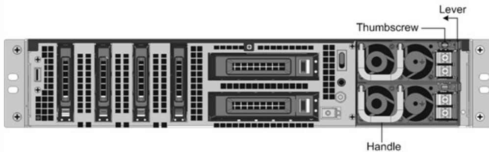
Figure 3. Removing the Existing DC Power Supply
