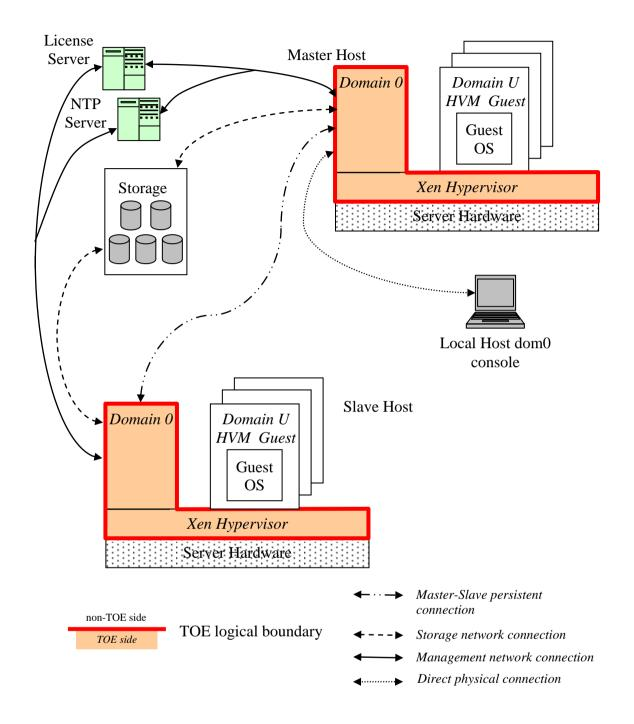
Figure 3: Illustration of TOE components and logical boundary
