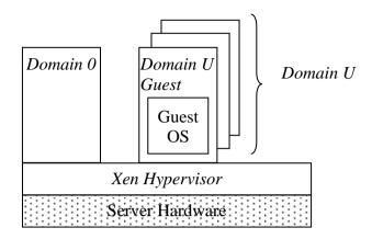
Figure 1: Illustration of XenServer components
