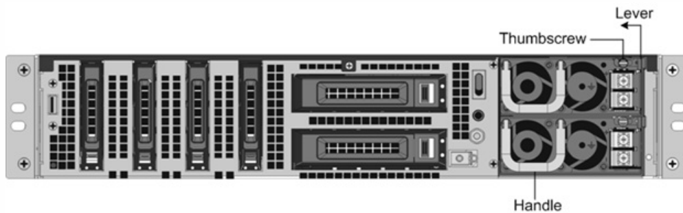
Figure 3. Removing the Existing DC Power Supply
