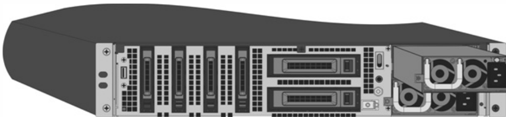
Figure 2. Inserting the Replacement AC Power Supply
