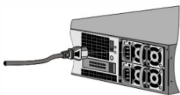
Figure 3. Inserting a power cable
