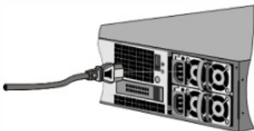
Figure 3. Inserting a power cable
