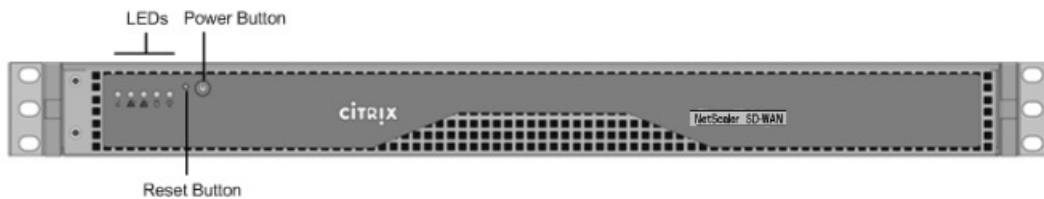
Figure 1. Citrix SD-WAN 1000 with Windows Server, front panel
