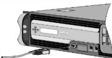
Figure 2. Inserting a console cable
