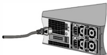
Figure 3. Inserting a power cable
