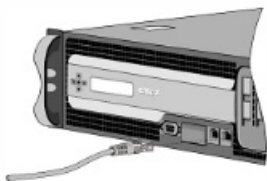
Figure 1. Inserting an Ethernet cable
