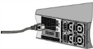
Figure 3. Inserting a power cable
