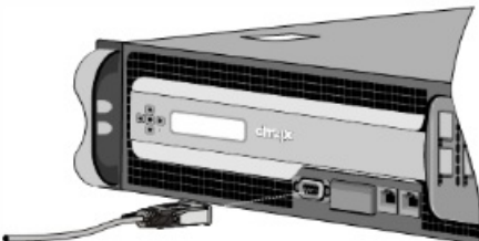
Figure 2. Inserting a console cable
