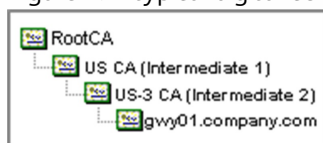
Figure 2. A typical digital certificate chain
