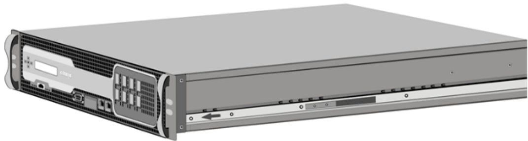
Figure 1. Attaching inner rails
