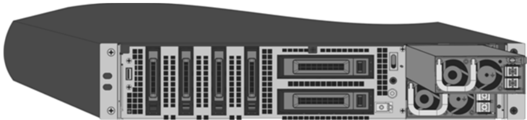
Figure 4. Inserting the Replacement DC Power Supply
