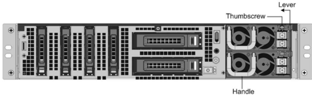
Figure 3. Removing the Existing DC Power Supply
