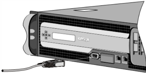
Figure 2. Inserting a console cable
