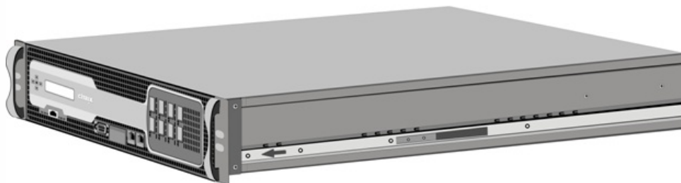
Figure 1. Attaching inner rails
