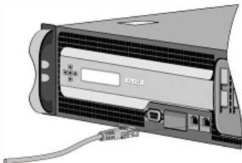
Figure 1. Inserting an Ethernet cable
