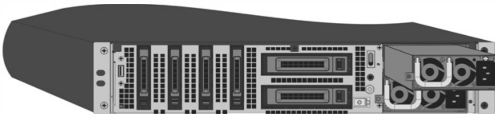
Figure 2. Inserting the Replacement AC Power Supply
