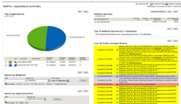
Application-specific flow information captured by AppFlow
