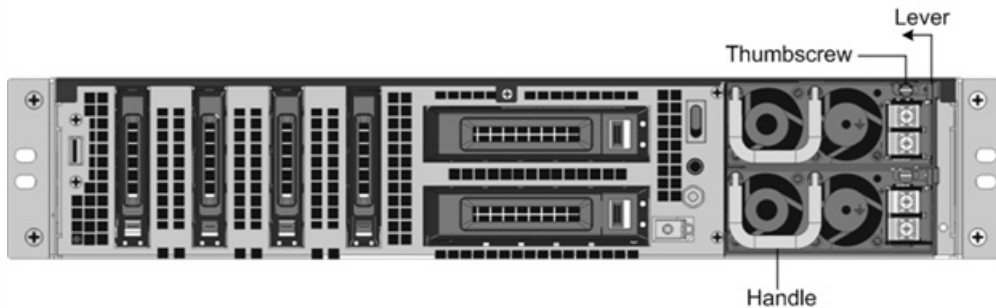
Figure 3. Removing the Existing DC Power Supply
