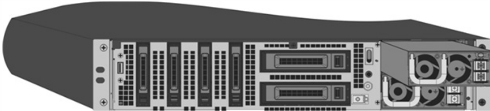
Figure 4. Inserting the Replacement DC Power Supply
