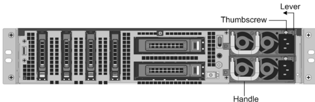
Figure 1. Removing the Existing AC Power Supply
