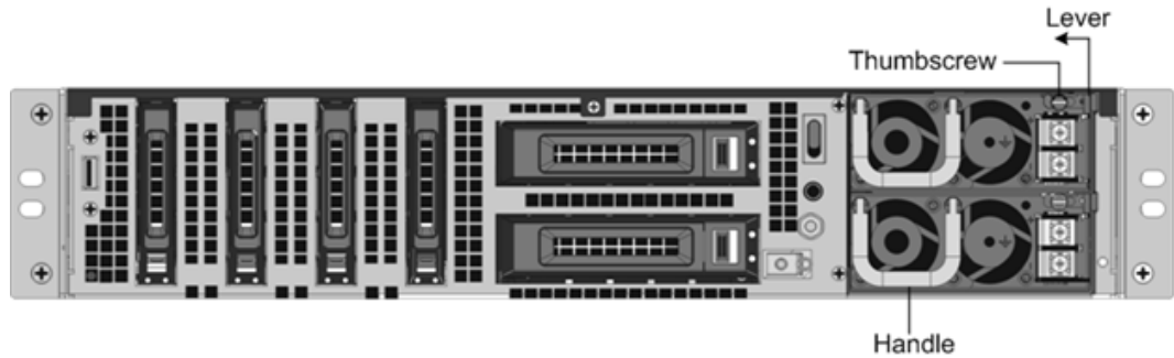
Figure 3. Removing the Existing DC Power Supply
