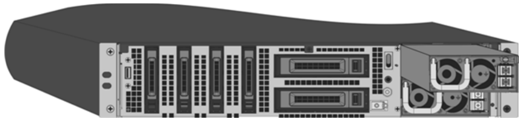
Figure 4. Inserting the Replacement DC Power Supply
