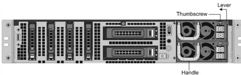
Figure 3. Removing the Existing DC Power Supply
