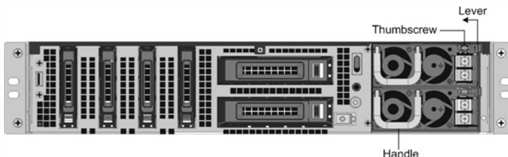
Figure 3. Removing the Existing DC Power Supply
