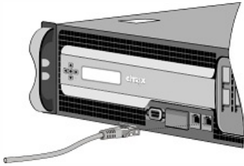
Figure 2. Inserting an Ethernet cable
