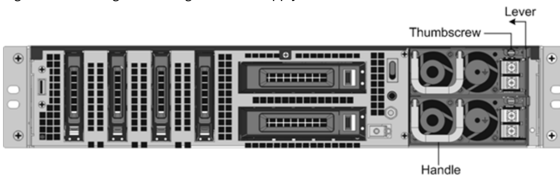
Figure 3. Removing the Existing DC Power Supply
