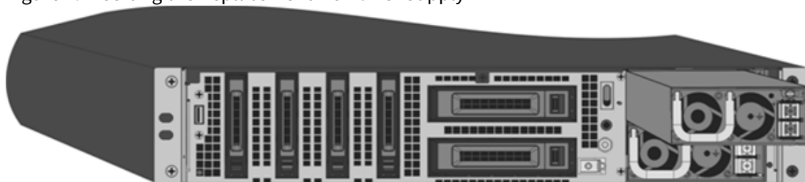
Figure 4. Inserting the Replacement DC Power Supply
