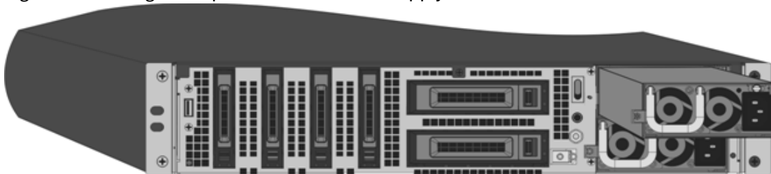
Figure 2. Inserting the Replacement AC Power Supply
