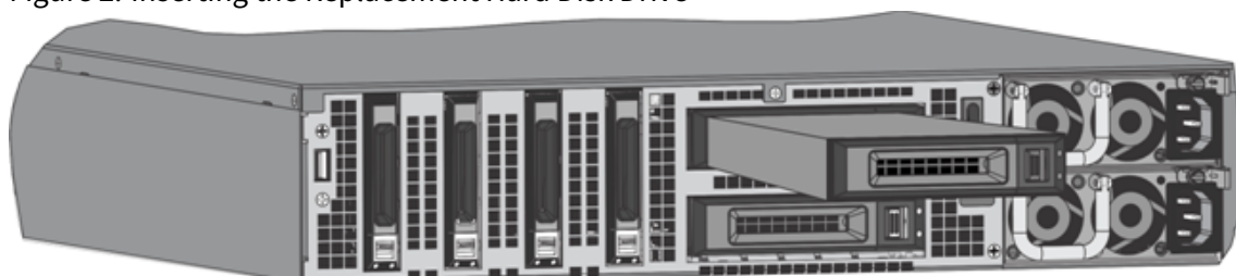
Figure 2. Inserting the Replacement Hard Disk Drive
