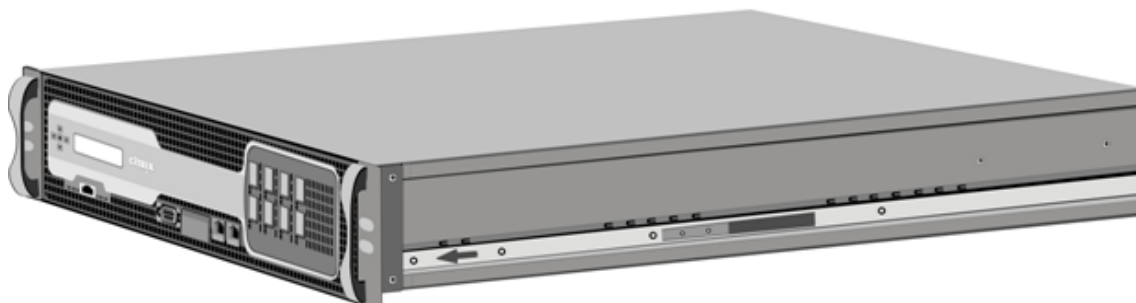
Figure 1. Attaching inner rails
