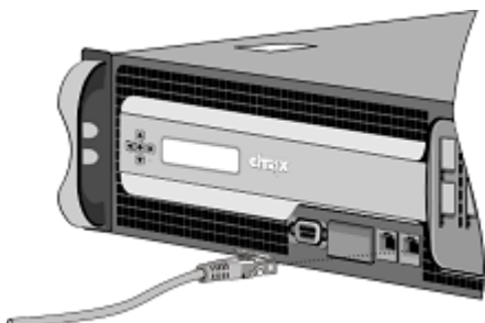
Figure 7. Inserting an Ethernet cable
