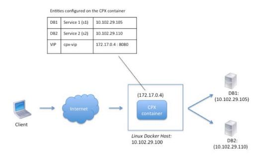
In this example, the Citrix ADC CPX container (172.17.0.4) sits between the client and the physical servers acting as a proxy. The servers, DB1 (10.102.29.105) and DB2 (10.102.29.110), reside outside a Docker host on the network. The client request originates from the Internet and is received on the Citrix ADC CPX, which distributes it across the two servers.
