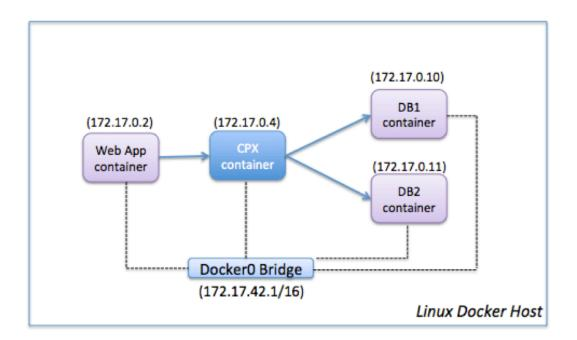
In this example, a web app container (172.17.0.2) is the client and the two database containers, DB1 (172.17.0.10) and DB2 (172.17.0.11), are the servers. The Citrix ADC CPX container (172.17.0.4) sits between the client and the servers acting as a proxy.
