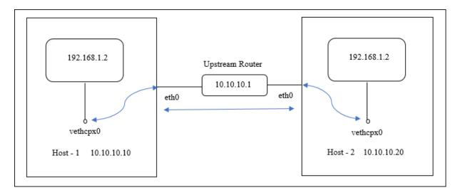
In this diagram, straight blue line represents flow of CPX-HA traffic between two hosts.
