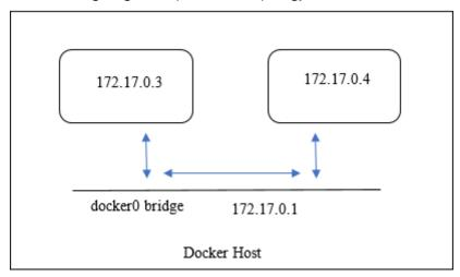
In this example two Citrix ADC CPX instances, CPX-1 (NSIP: 172.17.0.3) and CPX-2 (NSIP: 172.17.0.4), are created on the same Docker host. For high availability support, you must configure high availability nodes on both Citrix ADC CPX instances using the NSIP of the other node.
