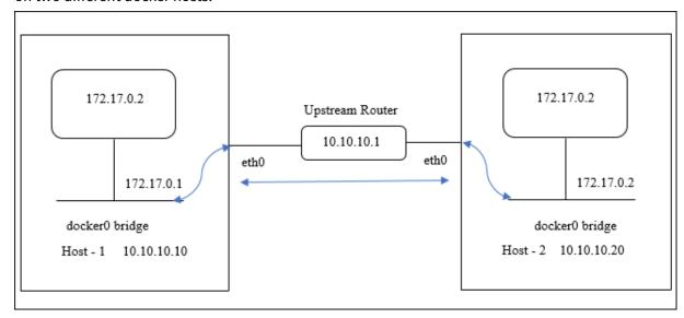
In this diagram, straight blue line represents flow of CPX-HA traffic between two hosts.
