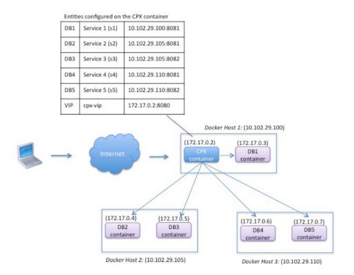
In this example, the Citrix ADC CPX instance and a server (DB1) are provisioned on the same Docker host with IP address 10.102.29.100. Four other servers (DB2, DB3, DB4, and DB5) are provisioned on two different Docker hosts, 10.102.29.105 and 10.102.29.110.
