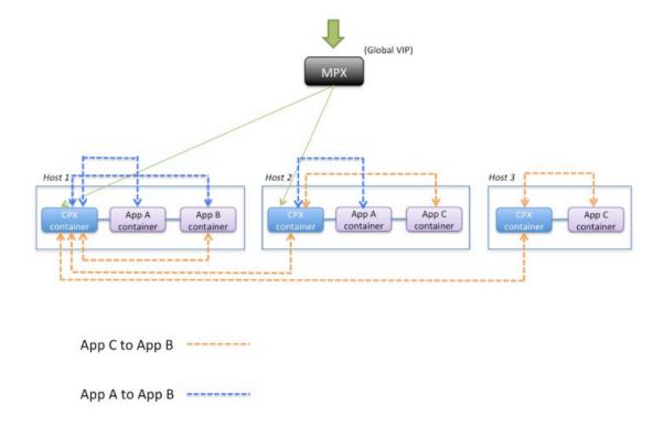
This image shows traffic flow between application C and application B and between application A and application B. When app C (in any of the hosts) sends a request to B, the request is first received on the Citrix ADC CPX container on the same host as app C. Then, the Citrix ADC CPX container passes the traffic to the Citrix ADC CPX container hosted on the same host as app B, and then the traffic is forwarded to app B. A similar traffic path is followed when app A sends request to app B.
